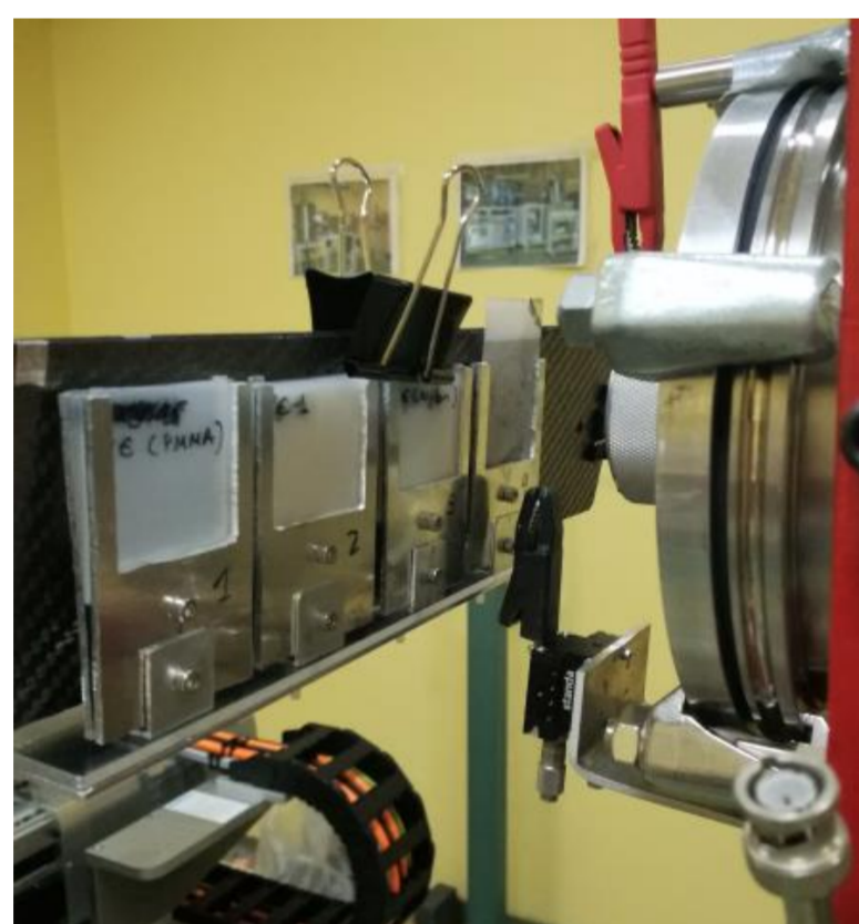
Fig. 4. Multi-layer targets made as a stack of thin ( \sim 200 \mu\text{m} ) films of PE ( \text{C}_2\text{H}_4 ), PMMA ( \text{C}_5\text{O}_2\text{H}_8 ) and Nylon-6 ( \text{C}_6\text{H}_{11}\text{NO} ) are mounted on a moving target holder in order to perform consecutive irradiations without accessing the bunker.
